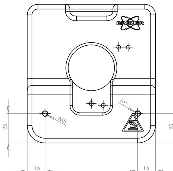
Fig. 4: Bruker Captive Spray Source with mounting holes
